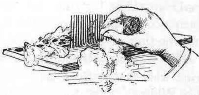
WHITNEY'S FIRST CONTRIVANCE FOR PULLING OFF THE COTTON SEEDS.
